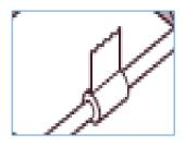
In the middle of this axle, wrap a small piece of tape to make a "catch" for the rubber band.
